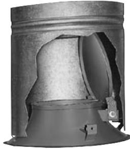
The damper is protected by an encircling windband. The damper is furnished with large hinge pins that rotate in oil impregnated bronze bearings for maintenance free operation.
