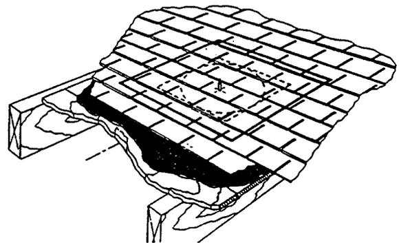
The nail is the center point; trace the outside of the fan base on to the roof shingles with chalk.
