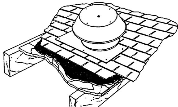
Slide ventilator under the shingles centering the fan over the hole; shingles should overlap the ventilator base flange on the upslope and the ventilator base should overlap the shingles on the downslope.
