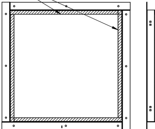
4) Attach adapter securely to wall (Fasteners not included. Depending on wall construction, this is to be attached at discretion of the installer.)
