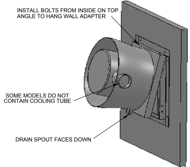
5) Hang fan from top bolts as shown; secure to wall adapter with remaining bolts.
