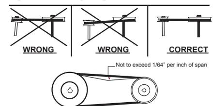
**CAUTION** *Whenever belts are removed or installed, never force belts over pulleys without loosening motor first to relieve belt tension. Before putting fan into operation, complete the following check list:*
