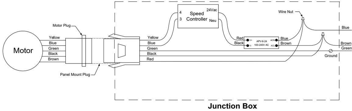
Figure 2: Internal Electrical Connections 208-230/277 V motor
