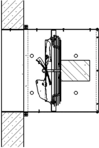
Figure 4: Typical Wall Sleeve and Damper Installation
