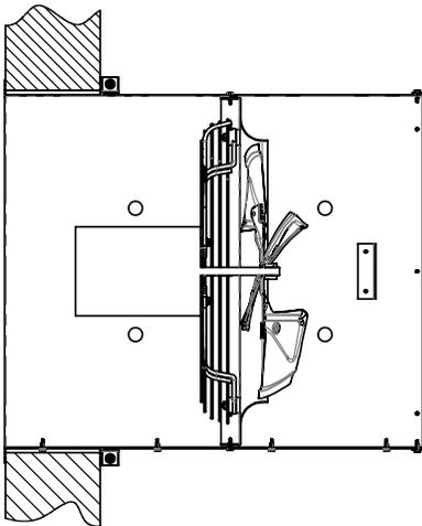
Figure 6: Typical Wall Sleeve and Damper Installation
