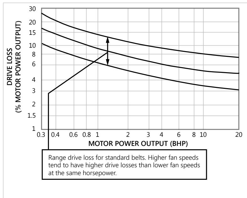
For totally enclosed, explosion proof, multi-speed and all 1.0 Service Factor motors, fan BHP plus drive losses should not exceed motor rated HP.
