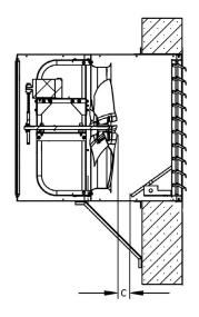
Figure 2: Fan Pack w/45deg weather hood
