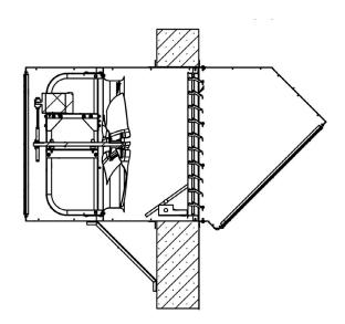
Minimum Clearance Between Fan and Damper – Figure 1 (example shown with a motorized damper)
